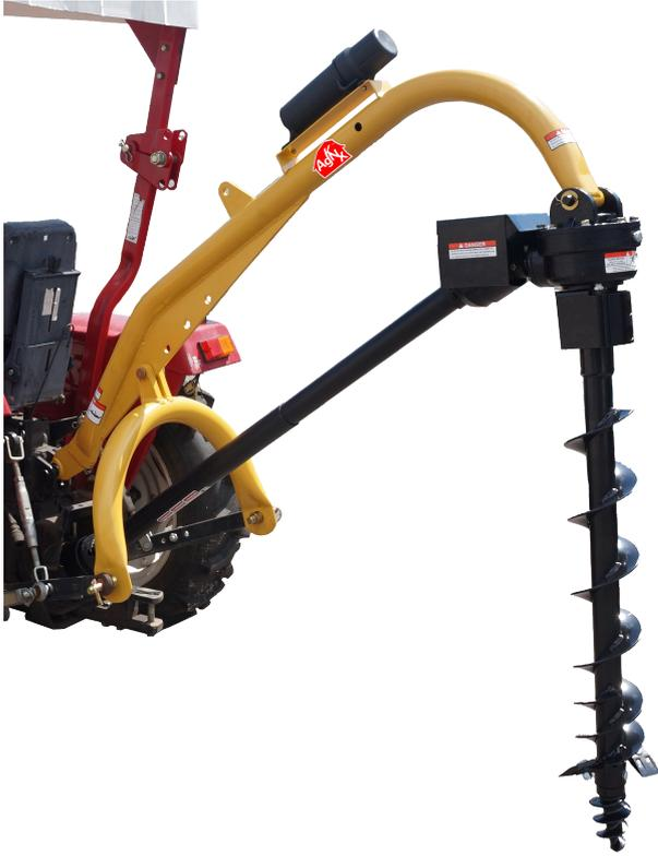
Post hole digger systems include a boom, A-frame, gear box, PTO driverline with safety shields, manual canister, all necessary pins and hardware kits. All models have an adjustable boom/A-frame connection. Diggers come in individual crate, which can fit one auger up to 9" and 12" depending on the model and crate ordered.
