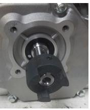
b. Place the spider on the engine coupler.
