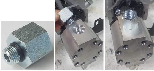
b. Install using an adjustable wrench the SAE-08 male to ¾" NPT male to the previous fitting. Lube up the o-ring on the fitting prior to installing. Place pipe tape on the ¾" NPT end after installing.
