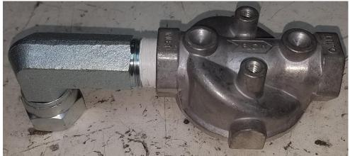
b. Apply pipe tape to the ¾" NPT to ¾" hose barbed 90 Deg fitting and thread it into the **outlet** of the filter base. The filter base can be on or removed at this point. The fitting should be facing down along the filter.
