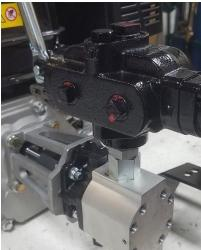
c. Rotate the valve mounting bracket and reinsert the 5/16" bolt, washer and locknut to secure the bracket to the pump, do not tighten.
