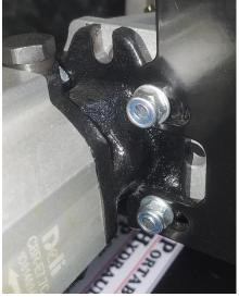
d. Using qty 2 M8-1.25 x 20mm screws, lock washers and washers, loosely attach the valve bracket to the valve. Any of the 4 threaded holes on the valve are acceptable. Use an M13 socket to tighten.
